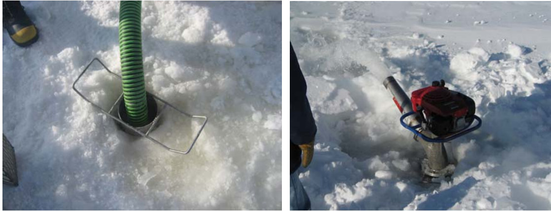
Fig. 3. Hanging basket screen in use with water truck and flood pump.
