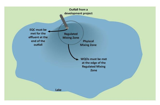
Figure 1a: Difference Between a Physical Mixing Zone and a Regulated Mixing Zone in a Lake
