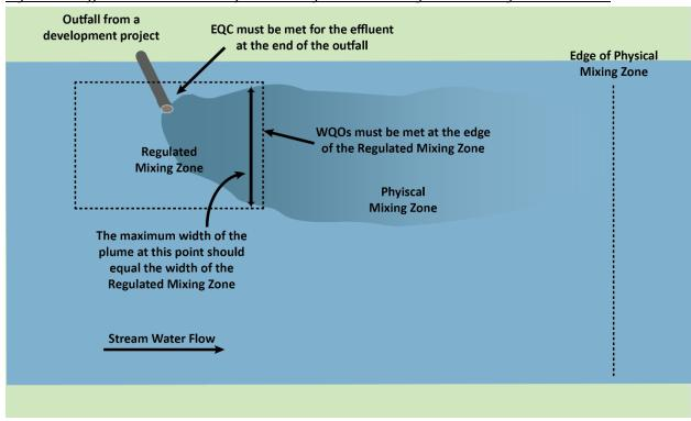
Figure 1b: Difference Between a Physical Mixing Zone and a Regulated Mixing Zone in a Stream
