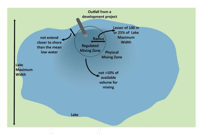
Figure 2a: Dimensions of a Regulated Mixing Zone for Lakes
