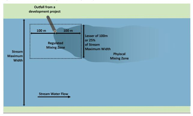
Figure 2b: Dimensions of a Regulated Mixing Zone for Streams or Rivers
