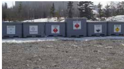
Figure 6-2: Containment for Various Waste Types
