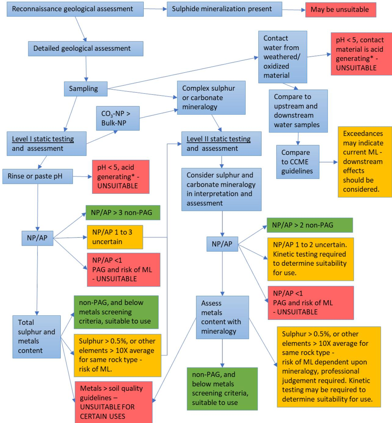
Figure notes: See text for further explanation of flow chart. \* = rinse pH or contact water pH of organic-rich surficial materials may be affected by organic acids, which are unrelated to acid generated from sulphide oxidation.
