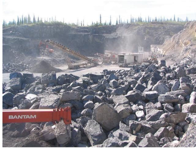
figure 22. Excessive dust caused by crushing operations can be mitigated by spraying water or using dust skirts on conveyors.
